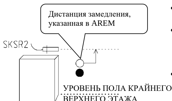
Figure-13: Installation of magnets for SKSR2
